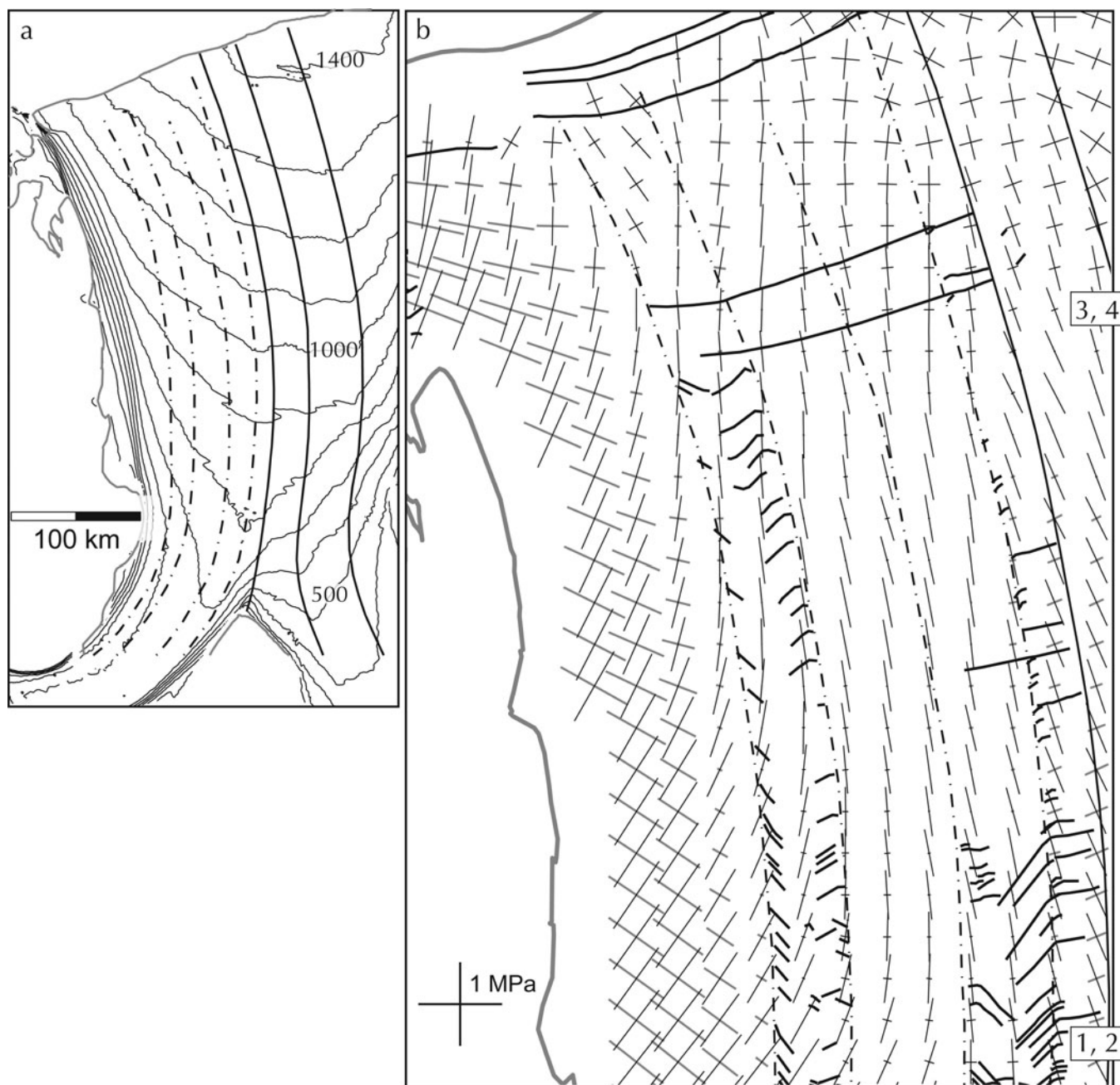
Fig. 4. (a) Observed surface speed, with contour interval 100 \text{ ma}^{-1} , and (b) computed principal deviatoric stresses in the EIS outflow. The contour interval is 100 \text{ ma}^{-1} . Lighter black curves in the stress map indicate extension, and heavier gray curves indicate compression. Sutures and fracture locations are from Figure 1. Locations of experiments described here are indicated by number.
